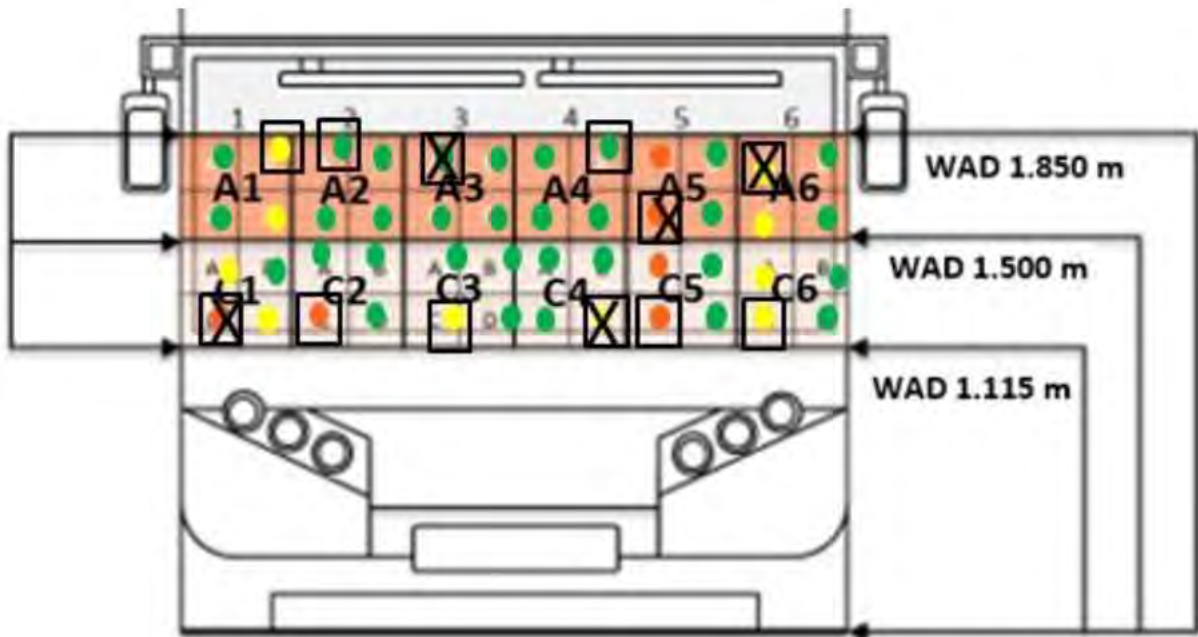
Figure 36_9: Example to illustrate simulation procedure; colour coded data supplied by manufacturer, selection of verification test points, and calculation of BITS value. Simulated test results shown by colour code, boxes identify the sub-areas with highest HIC15 within the twelve test areas and crosses identify test points for chosen verification tests
